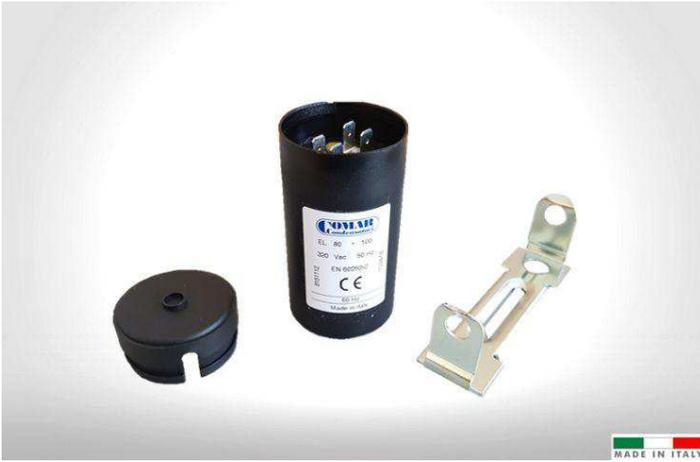
The **EL** electrolytic capacitor have **high capacitance** ( $\mu\text{F}$  value) able to provide an high starting torque to the motor. It is a non polarized capacitor especially designed for intermittent AC voltage applications for single-phase motors.
