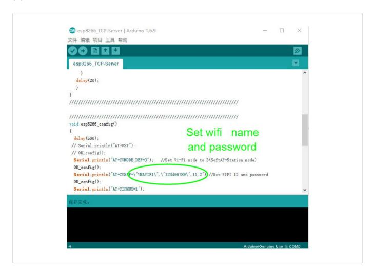
Compile and upload this code to your Arduino<sup>®</sup> UNO. Please note during the uploading progress, to turn the switch to "off" and to turn to "on" when the uploading is finished. When it is done, you can open your cell phone WiFi to check if there is a WiFi named "VMAWIFI".
