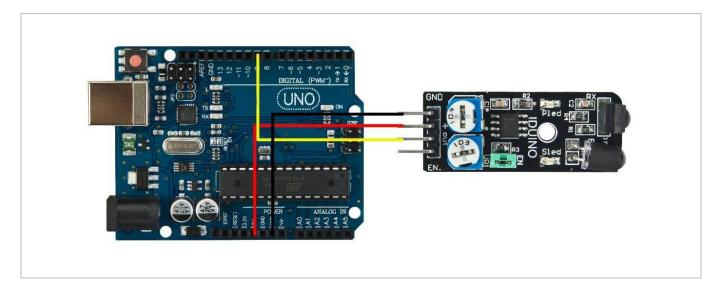
Tip: The VMA330 can be used as an IR remote-control tester as well! Point any IR remote control towards the VMA330 and you will see the SLED flashing when the remote is working.
