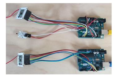
We will connect two radio modules to one another, read the temperature and send the temperature value to another module.
