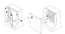
To install or replace the filter in the fume extractor, proceed as follows:
