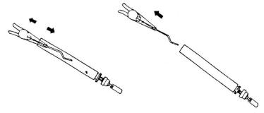
**6.** Clean the cooling strip and collector with a wire brush (included).
