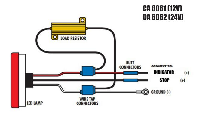
Insert Wires, squeeze with pliers to snap, splice tap shut - Do not cut your vehicle Wires
