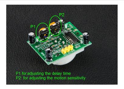
RP1 = adjustment for delay on time
