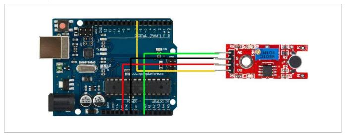
In this example, we try to combine the digital and analogue pin in order to control two LEDs. Connect as above.
