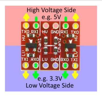
To send a signal from the low-voltage side to the high-voltage side (e.g. from 3.3 V to 5 V), the signal must be input at TXI. It will pass through the converter and come out as a higher voltage on the TXO (transmit output) pin.
