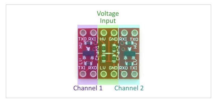
The middle section of the board serves the high and low voltages. Supplying voltage to all four of these pins is required.
