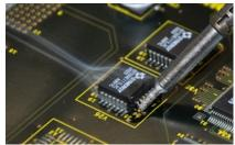
Efficient solder fume extration directly at the solder joint
