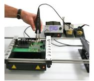
SMD desoldering with the CHIP TOOL desoldering tweezers. Bottom-side preheating with heating plate provides for gentle processes.
