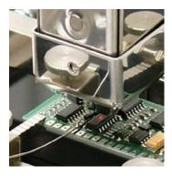
Temperature-controlled SMD soldering
