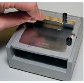
Flux application in a dip stencil
