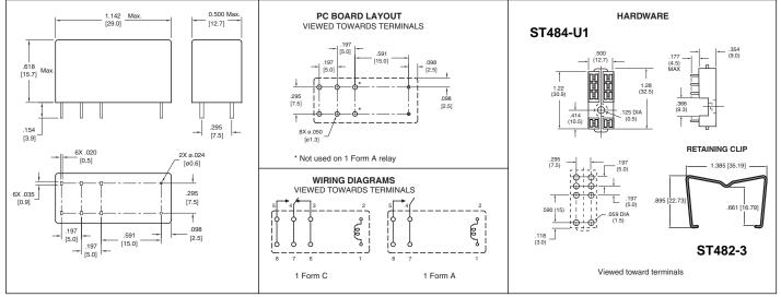
Dimensions in inches with metric equivalents in parentheses. Tolerance: ± .010"
