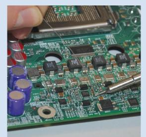
The soldering tip is the "heart" of the soldering iron and responsible for the heat transfer from the heating element via solder to the solder joint.
