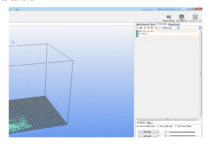
Now select "Final G-code", enter G01 X0 Y0 F500; back to X0 Y0 position with linear movement of 500 mm/min and save it.
