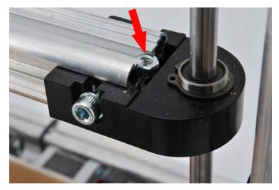
The next operation concerns the displacement of the extruder from the original position. The extruder is fixed to a bracket which, in turn, is attached to the horizontal printer arm using 2 M5 screws. Before moving, make a mark with a pencil on the printer arm at the centerline of the bracket that holds the extruder (to allow in the future to relocate the extruder in the correct position). Cut and remove the plastic clamps that secure the wiring to the arm.
