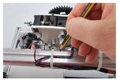
Unscrew with an allen key and remove the 2 screws that fasten the bracket to the arm.
