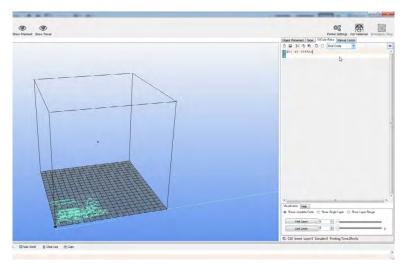
These changes are needed to define the offset of the coordinate system so that the machine operates in the desired area and back to the starting point when processing is finished.
