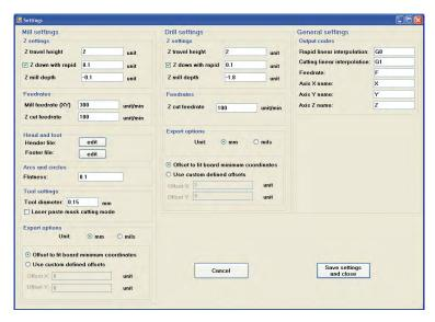
The first part "Mill settings" allows you to set some of the parameters required for the creation of the G-Code related to the incision of the tracks, such as feedrates, mill depth, etc. We recommend to keep the parameters we show (visible in the picture above). The only thing that you have to set is the tool diameter that depends on the mill (chisel) that will be used (in our case 0.15mm).
