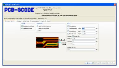
In the "Generation Options" folder check the two entries under "Top Side" and the entry Single pass of "Isolation". This allows to make tracks patterning with a single pass of the tool.
