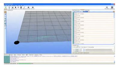
Pick up few inches the Z-axis by acting on the manual control keys (be careful not to move X and Y!) and replace the chisel with a drilling bit of suitable diameter (e.g. 0.8 mm).
