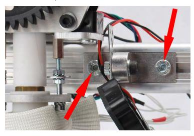
Move the extruder over the arm completely to the left (as shown in photo). Move to the same side also the fan.
