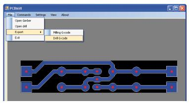
The file generated by PCBMill visible in the image below must be imported into G-Code Editor of Repetier – Host (with a simple copy and paste).
