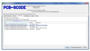
The folder "GCode Options" allows to choose whether to insert comments in the generated G -code (in our case do not check any item), if use a custom G -code and more. In the creation of our PCB we just ticked off the entry "Use simple drill code" (which allows to get a drilling G -code compatible with Repetier - Host) and called "nc" as Extension (always to make the generated files compatible with Repetier - Host). The last 2 folders (Plugins and Other) were not taken into account.
