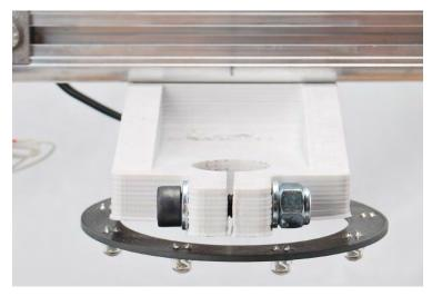
Place the power tool in the collar and, after fixing to the plastic stand, insert any bit in the mandrel and verify that, in HOME position, there is no contact between the tool and the work surface.
