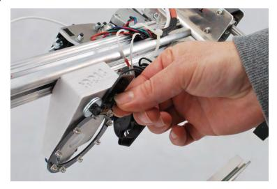
Before tightening the screws, place the bracket of the electric mandrel with the centerline moved about 1 cm to the left compared to the benchmark, reported in pencil on the arm, so that during the HOME, the position of the electric mandrel turns out external to plate, thus avoiding eventual collisions with the tool.
