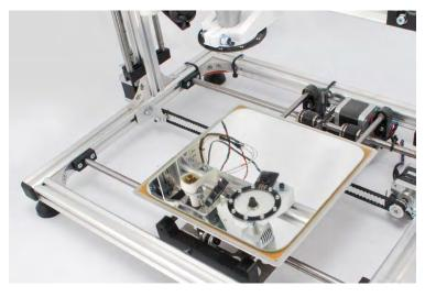
Attach to the glass / mirror a "sacrificial" plan of suitable thickness (about 1 cm) in order to drill the holes of the PCB without damaging or breaking the tool. That plan could be MDF, forex, plywood, etc. ... no humps, bumps or other deformations.
