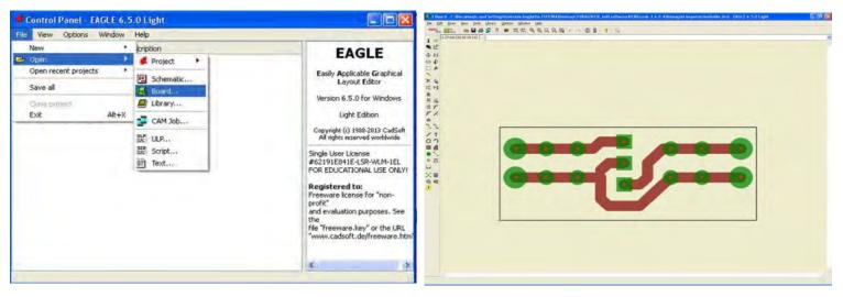
Mirror the printed circuit board and align the lower left corner of the base with the starting point of the worksheet. This operation is to keep the PCB in the work plan and to orient the PCB so that the copper side to work (called "Bottom Copper") is facing upwards.
