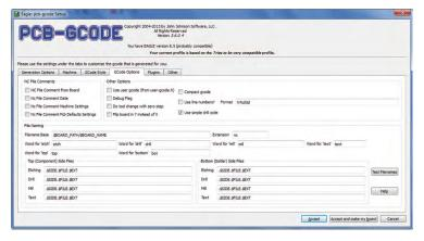
After setting PCB- gcode parameters, click Accept to confirm your choices (the setup window will close and on the monitor the Board Editor screen with its own PCB will reappear). To create the G -code files useful for tracks etching and base drilling, type in the appropriate field run pcb-gcode-setup and press enter.
