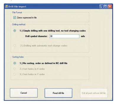
Load the file relating to holes of the PCB whose tracks patterning has been carried out by milling (e.g. Drill Data.drl). The software will automatically create the corresponding G-Code showing the holes that will be made with red dots.
