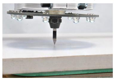
Attach the strip copper to work on the sacrificial level, with the double-sided tape.
