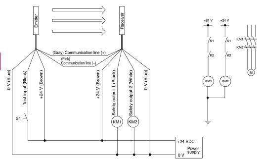
S1 : External test/lockout reset switch (connect to 0 V if a switch is not required)
