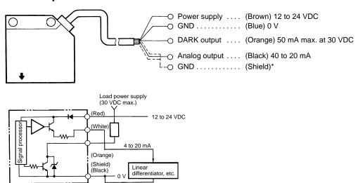
Note: 1. \*The two ground terminals (black and shield) are internally connected. However, the black ground must be used with the red terminal for the power supply and the
