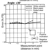
Note: The LED Displacement Sensor cannot detect an object accurately if the object is positioned at an angle oblique to the sensor position. If the oblique angle is large, detection is not possible because of insufficient reflection of light. This must be taken into consideration when installing the sensor.
