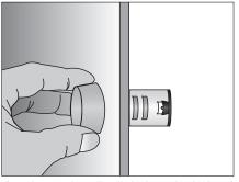
Just insert the pilot light into the hole of the pannel.
