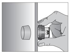
The pilot light will be secured at the The pilot light has been installed. back by the plastic nut
