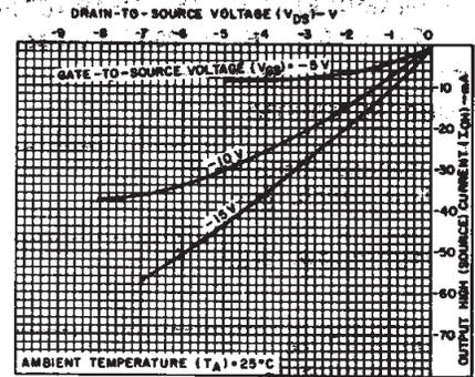
Fig. 4—Typical p-channel output high (source) current characteristics.
