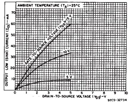
Fig. 2—Typical n-channel output low (sink) current characteristics.
