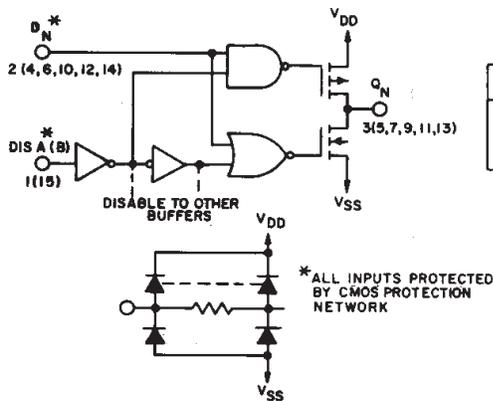
Fig. 1—Logic diagram of 1 to 6 identical buffers.
