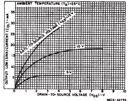
Fig. 3—Minimum n-channel output low (sink) current characteristics.
