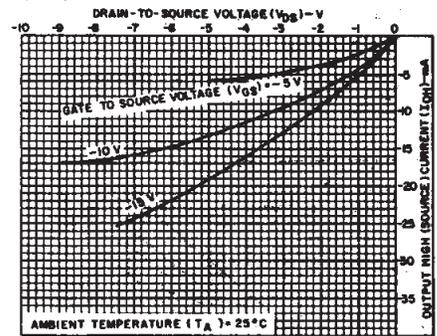
Fig. 5—Minimum p-channel output high (source) current characteristics.
