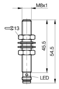
Inductive Sensors BES 516-324-G-S 49-C M8x1 x 54.5 normally-open Sn=2mm shielded
